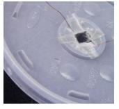
The final voice coil should look something like this with the glue flanges on the outside and the coil extending into the cup or bottle.
