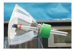
The magnet is inserted into the coil and the diaphragm is secured in place. Slide the magnet support forward so the magnet is in the coil. Do not insert too far or the coil will hit the wire tie.
