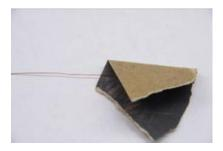
Be sure to remove the insulation from the wires. It is best to use some fine sandpaper or emery cloth.
