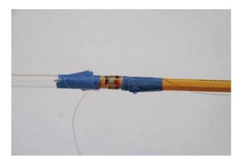
You will need several layers and always wrap in the same direction. Try to wrap uniformly. Once the coil is completely wound; cut off the remaining straw so that the edge of the coil is near one end of the
