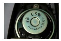
Do not try to connect a low impedance speaker to the headphone jack. Head phones are very high impedance devices and the speaker will load down the circuit. If you want to drive the Soda Bottle speaker from a headphone jack, it is best to use an amplifier. If you have a set of amplified computer speakers, you can use a Soda Bottle or Cup speaker to replace the actual speaker inside of the housing. As you can see, I have use Soda Cup speaker to replace one of my amplified computer speakers.
