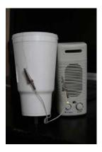
The Cup Speaker replaces my normal left speaker. I have also clipped a lead from the right speaker in the amplifier housing. That way I only hear the left speaker (Cup). This amplified speaker can now be plugged into any headphone jack without causing an impedance mismatch. You can use it with you tablet, mp3 player or other portable devices.
