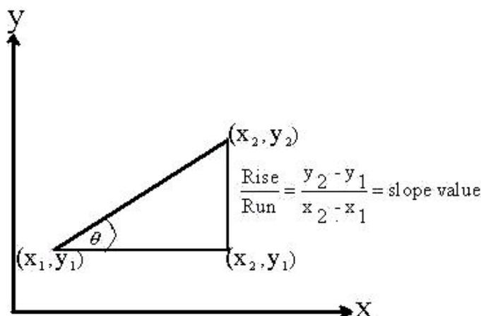
Figure 1: Determination of slope value using the rise-over-run method.
