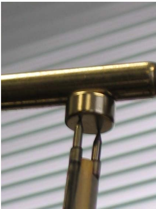
Figure 2. Axis comprising a pair of replacement ball-point-pen inserts supporting the pendulum and hanging from a rare-earth magnet.
