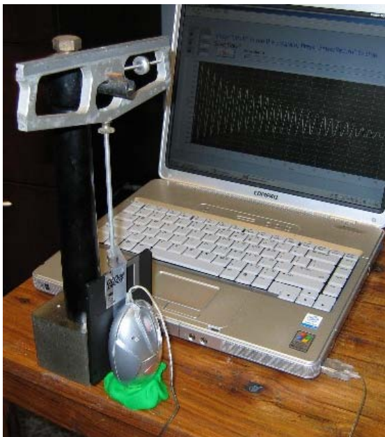
Figure 1. First pendulum that was tested. The mouse is held in place with play-doh.
