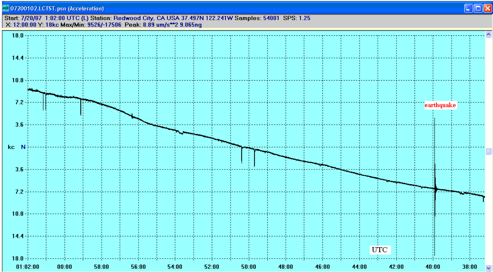
Figure 2. Pulses observed before the earthquake of 20 July 2007 near Oakland CA, by a VolksMeter seismograph situated in Redwood City, CA. In this 12-h total duration record, the first pulse occurs more than 10 hours before the Mw 4.2 earthquake.
