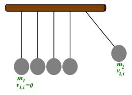
Conservation of Momentum  $m_1 v_{1,i} + m_2 v_{2,i} = m_1 v_{1,f} + m_2 v_{2,f}$  if  $m_1 = m_2$  then  $v_{1,f} = v_{2,i}$ ,  $v_{2,f} = 0$
